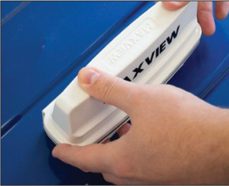
9. Fit the Roam Antenna to the Bracket - Press firmly around the edges of the antenna to ensure a watertight seal has been achieved
